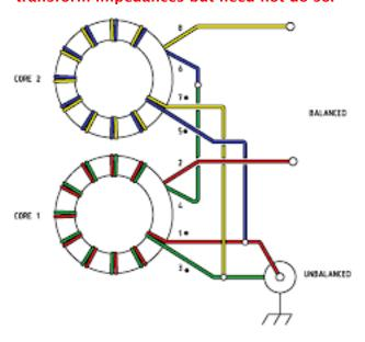
Although widely used with RF antennas, baluns may also be used in a variety of applications including: power line communications; data communications converting between Cat 5, Cat 6, etc and Twinax; video where a conversion between a twisted pair and a coaxial cable, etc. There are many other uses for baluns, but these are some of the main ones.
